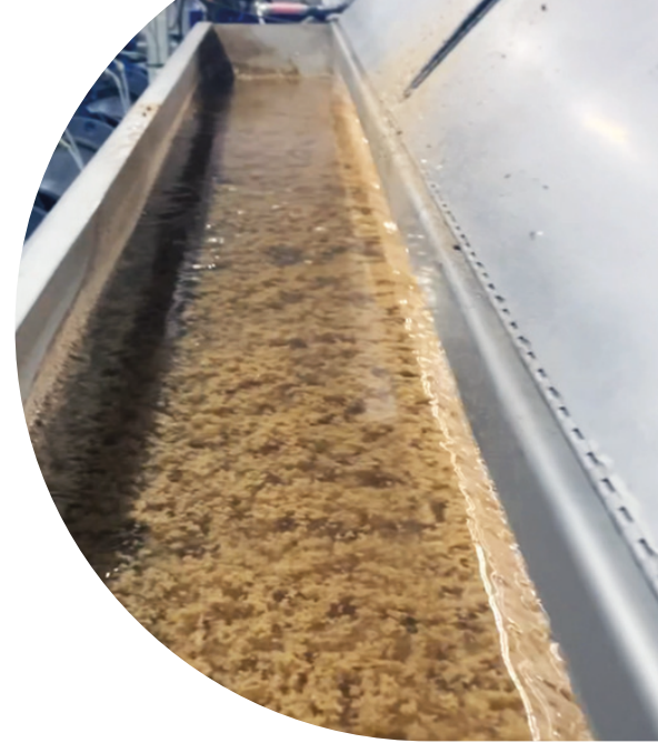
High DM wastewater – strong flocs.
