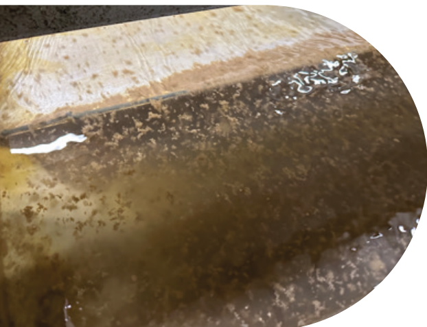
Low DM wastewater – strong flocs.
