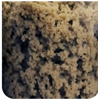
Picture 5. Left beaker (picture 4) added approx. 50 ppm with PAM. Strong flocculation and good phase separation.
