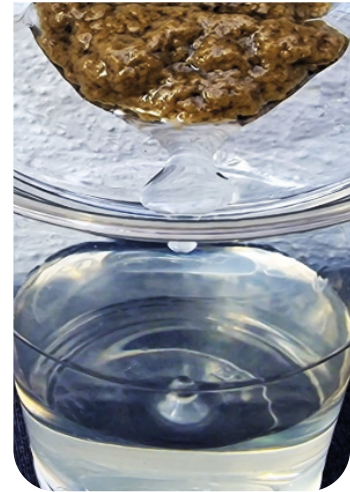
Picture 6. The flocculated sludge drains the water phase effectively.
