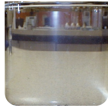
Picture 3. Middle beaker (picture 2) a few seconds after stopping stirring. High sinking speed provides efficient separation.
