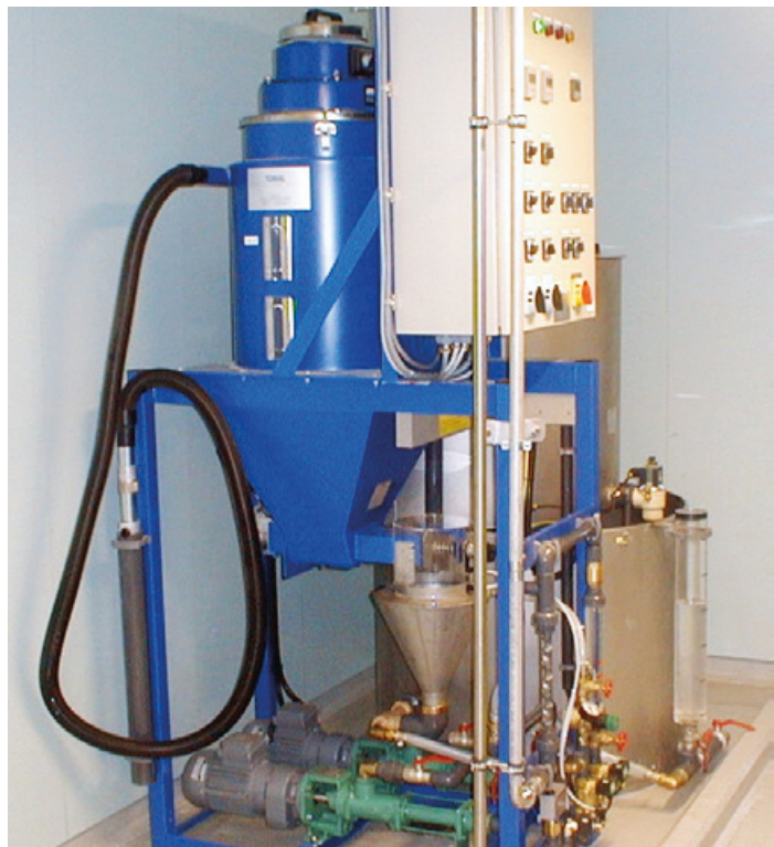
Example of polymer preparation device for powder PAM.
