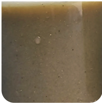
Picture 4. Untreated O sample (organic sludge) Dry matter approx. 4-5%. Very difficult to separate dry matter from water.
